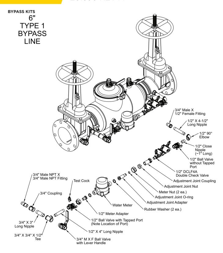
APPLY TEFLON TAPE TO PIPE THREADS AND INSTALL COMPONENTS AS SHOWN.
