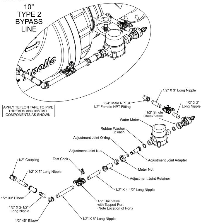
APPLY TEFLON TAPE TO PIPE THREADS AND INSTALL COMPONENTS AS SHOWN.
