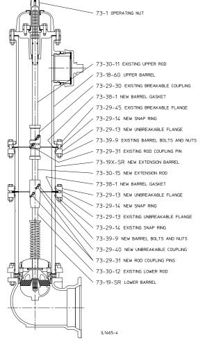
NOTE: The use of extension lengths made by more than one extension kit is not recommended. When combined extension kit and existing trench depth exceeds 9 ft, replace existing lower rod with appropriate length lower rod instead of using rod extension. When combined length exceeds 12 ft rod guides are recommended for lower rod.
