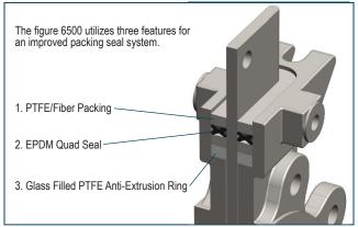
In addition to the curved packing chamber, the figure 6500 knife gate valve standard packing configuration includes:
