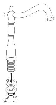
3. Set the spout into the center faucet hole. Position the decorative escutcheon so that the hole for the drain's lift rod is in the back.
