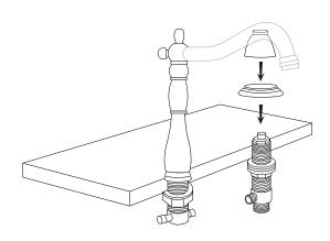
8. From beneath the sink, position the stem so that the outlet on the side of the stem is pointing inward, towards the T-connector. While holding in place, hand tighten the lock not. Finish tightening using a basin wrench.
