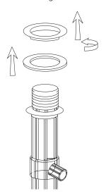
2. Set the flat rubber gasket over the drain hole in your sink, then insert the flange into the drain hole.
