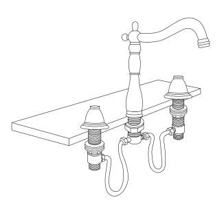
11. Attach the main water lines to the proper inlet on the bottom of each valve stem. Use an adjustable wrench to tighten, but be careful not to overtighten. Apply thread sealant or plumber's tape to each threaded connection. Ensure that you are connecting the hot and cold lines appropriately.
