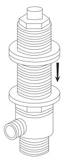
7. From under the countertop, insert the valve stem into the right-side faucet hole. From above the counter top, slide one of two decorative escuthceons onto the stem. Then, attach one of the two bell flanges to the stem by hand tightening until secure.
