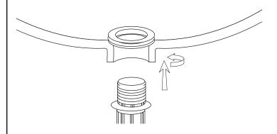
4. Connect the drain lever by threading it into the hole on the side of the drain body. The lever must pass through the hole in the stopper tailpiece to function properly. Apply a bit of thread sealant or plumber's tape to the threads before attaching.
