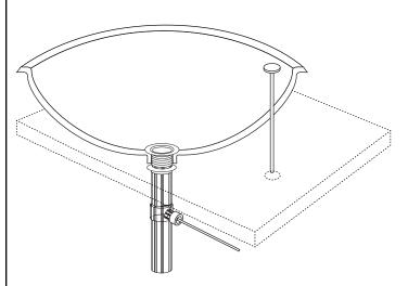
7. Use the link to attach the faucet's lift rod to the drain lever. Pinch the metal clip located on the drain lever to remove. Slide one end of the clip back onto the lever, followed by the link, then the second end of the clip to secure.
