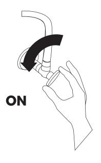
6. Remove the aerator from the spout and turn the faucet on to remove any dust or loose sediment from the water lines. Check for leaks. Check to ensure that both hot and cold water are running properly. Allow the water to flow for approximately 60 seconds, then reattach the aerator.
