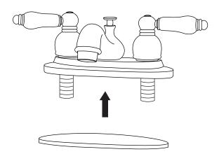
3. Insert the faucet into its prepared mounting holes. From below, secure the faucet by tightening the provided lock nuts onto each threaded shank. Hand tighten firmly. Finish tightening with an adjustable wrench if desired.
