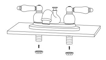
4. Connect the main water supply lines to the threaded shanks of the faucet. If needed, use the provided cone washers and lock nuts to make the connections. Apply thread sealant or plumber's tape to the threads before attaching.
