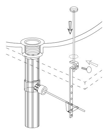
9. Make any final adjustments to the positioning of the link and drain lever as needed. Adjust until the drain fully opens and closes.
