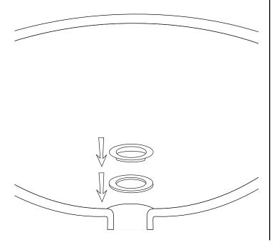
3. From beneath the sink, reattach the flange by threading it back onto the drain body.
