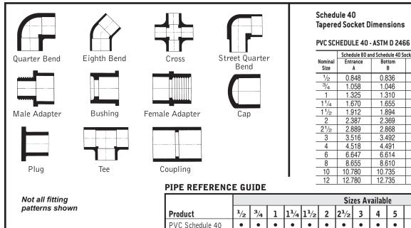
Schedule 40 Schedule 80 and Schedule 40 Socket Diameter Schedule 80 Tolerance Socket Length Socket Length C (Minimum) C (Minimum) 0.836 ±0.004 0.875 0.688 1.046 ±0.004 1.000 0.719 1.310 ±0.005 1.125 0.875 1.655 ±0.005 1.250 0.938 1.894 ±0.006 1.375 1.094 2.369 ±0.006 1.500 1.156 2.868 ±0.007 1.750 1.750 3.492 1.875 1.875 ±0.008 4.491 ±0.009 2.250 2.000 ±0.011 3.000 6.614 3.000 8.610 ±0.015 4.000 4.000 10.735 ±0.015 5.000 5.000 6.000 12.735 ±0.015 6.000
