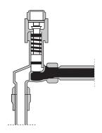
Locked closed for hydrostatic test
