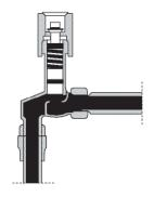
Manual Open: Drain or flow switch test
