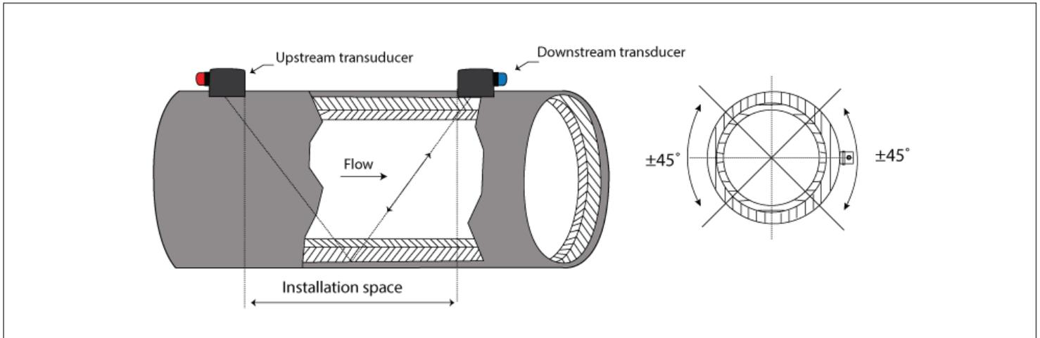
The V method is a standard installation method and convenient to use for precise measurement of flow. While installing the two transducers, they are horizontally aligned. The transducers center lines are parallel with the pipe axis line. They are suitable for pipe diameter range  $\frac{1}{2}$ " to 16" (DN15 mm-DN400 mm).
