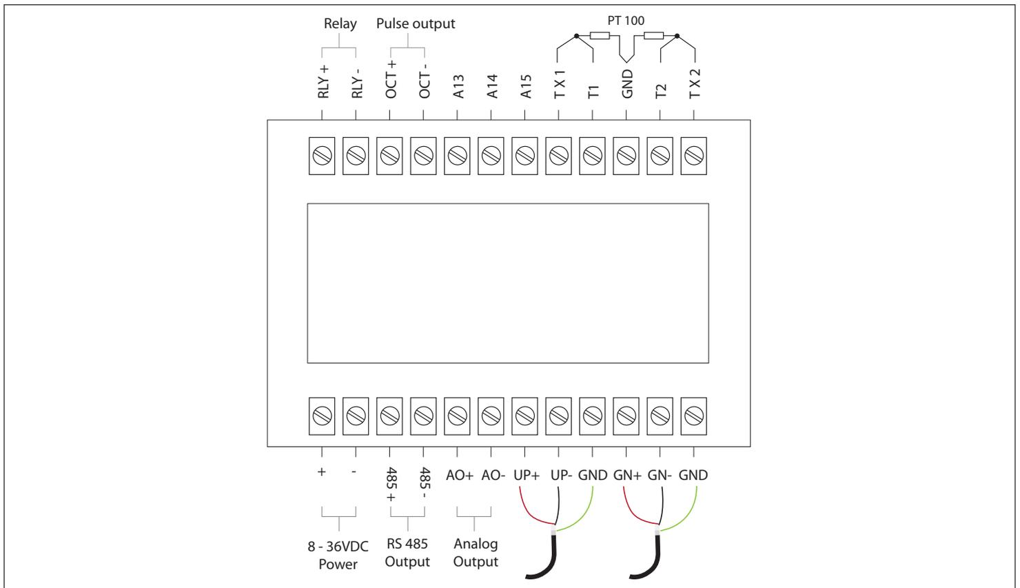
● Signal Wiring Diagram of 1200A-100EXP
