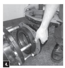
Lubricate new Shoe and Bottom Seat Ring O-ring. Position Shoe to slip in place.
