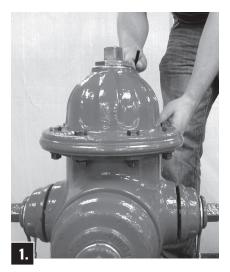
Remove Oil Filler Plug and check oil level. Oil should be level with Oil Filler Plug Hole.
