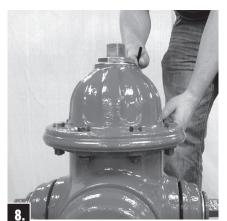
Remove Oil Filler Plug in side of Bonnet. Pour MUELLER Hydrant Lubricant into Oil Reservoir until it is level with Oil Filler Plug Hole. Replace Oil Filler Plug (see Lubrication section on page 8).
