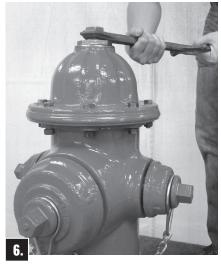
Turn Operating Nut in closing direction to make sure Main Valve is closed tightly, then turn in opening direction approximately 1/4 turn to relieve tension on operating mechanism.
