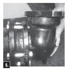
Slip new Shoe in place being careful not to damage Bottom Seat Ring O-ring.
