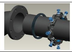
4. Insert the O-Ring into the groove of the Adapter ring if this is provided separately, if not make sure the O-Ring is in the correct position in the groove. Slide the Adapter Ring on the pipe with the O-Ring facing the plain end of the pipe and the gasket recess facing either the Sigma Seal gasket or transition gasket and restrainer gland.
