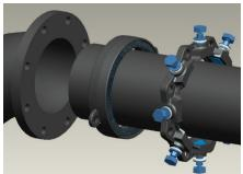
5. Join the pipe-end and flange together within the maximum assembled deflection and maximum allowable gap "L" to the flange face. Slide the adapter ring, gasket and restrainer gland until contact is made with the opposing flange.
