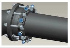
NOTE: WHEN USING SIGMA FLANGE UNIVERSAL JOINT WITH HDPE PIPE A PIPE STIFFENER/INSERT IS RECOMMENDED TO BE USED AND PLACED DIRECTLY BELOW THE POSITION OF THE WEDGE RESTRAINING GLAND.
