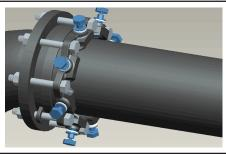
8. If removal is necessary, loosen the actuating wedge bolts using the remaining hex shank. To re-install the joint, repeat steps 2 through 7 and torque the hex shanks to the specified value.
