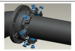
7. Hand-tighten the break-off bolts in an alternating manner (star pattern) until all wedges are in contact with the pipe surface. Tighten the heads in an alternating manner (star pattern) until the heads are sheared off.
