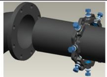
3. Lubricant the plain-end of pipe and gasket, then slide the Sigma Seal gasket onto the pipe. (Transition gasket needs to be used for Steel & IPS OD PVC pipe.)
