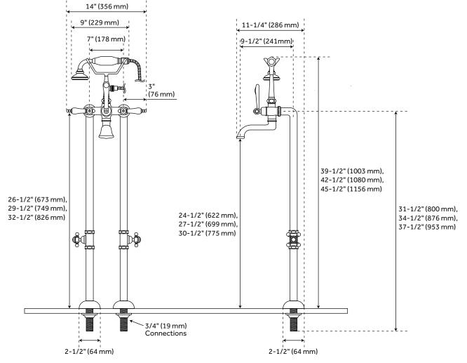
Underfloor access is required for proper installation. Installation on a concrete slab will require cutting and concrete removal.
