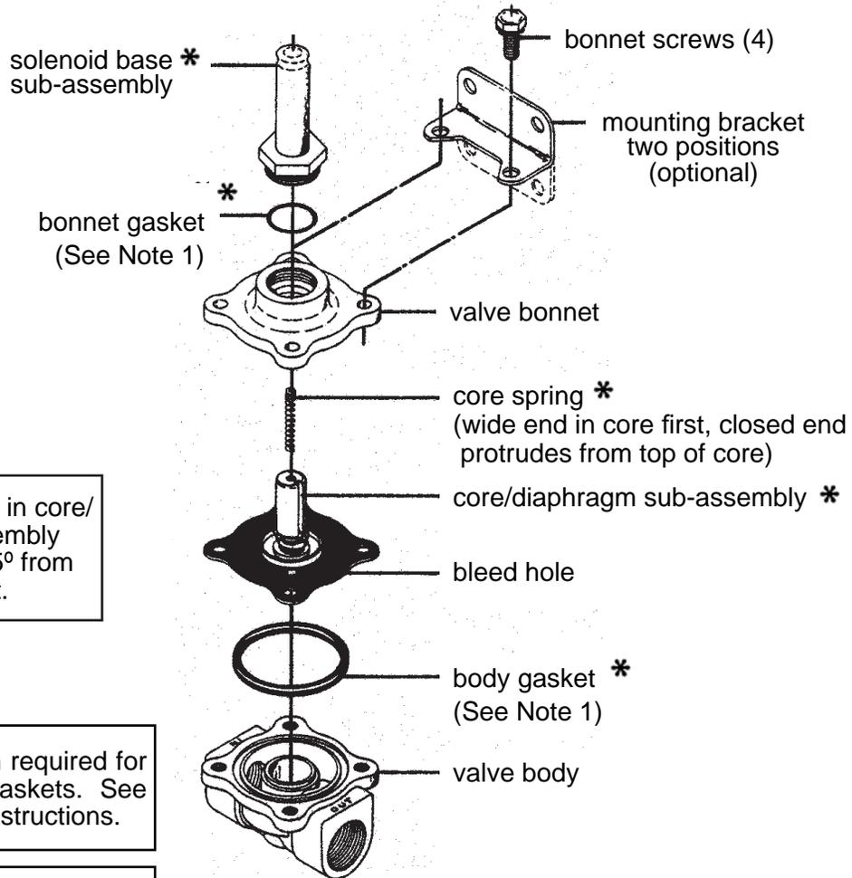
Locate bleed hole in core/diaphragm assembly approximately 45° from valve outlet.
