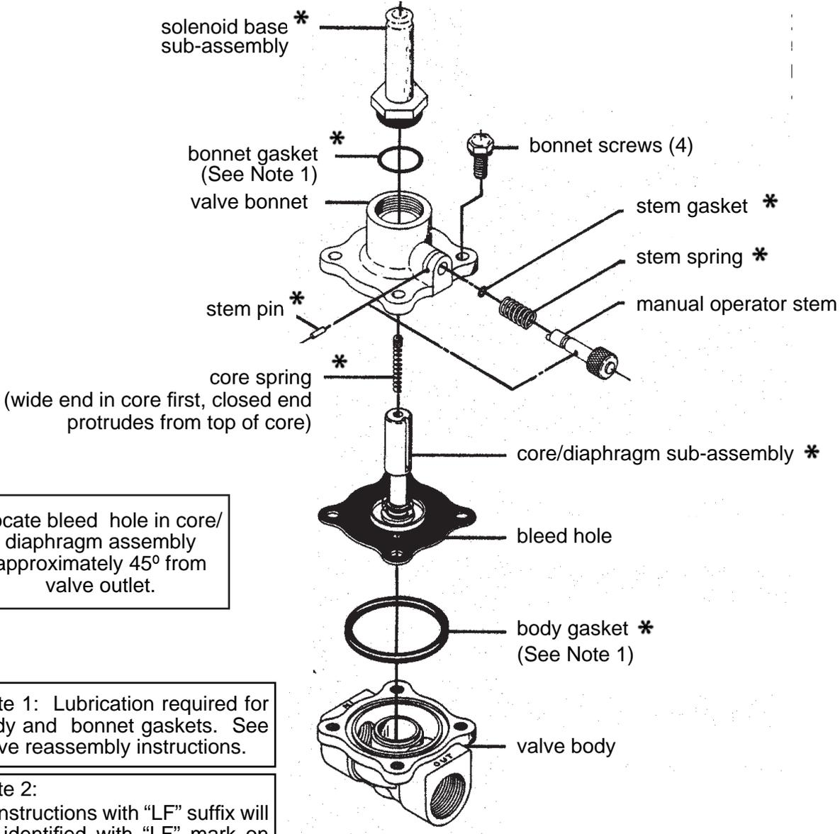
Locate bleed hole in core/diaphragm assembly approximately 45° from valve outlet.
