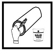
Step 4: Apply "Blue Lube" liberally to the spigot of pipe. Keep the lubricated surfaces free from dirt.
