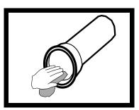
Step 1: Clean bell of pipe. Remove any loose dirt, gravel, rust, scale, or foreign material. Remove standing water for best results.
