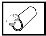
Step 2: Clean spigot of pipe as in Step 1. Surfaces must be thoroughly clean before application of "Blue Lube".
