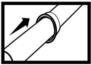
Step 5: Immediately after application of the lubricant, assemble the joint. Apply even pressure and insert the spigot into the bell.
