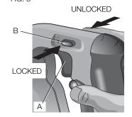
**AWARNING:** This tool has no provision to lock the switch in the ON position, and should never be locked ON by any other means.
