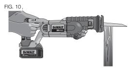
**ÀWARNING:** Use extra caution when cutting overhead and pay particular attention to overhead wires which may be hidden from view. Anticipate the path of falling branches and debris ahead of time. **ÀWARNING:** Inspect work site for hidden gas pipes, water pipes, or electrical wires before making blind or plunge cuts. Failure to do so may result in explosion, property damage, electric shock, and/or serious personal injury.
