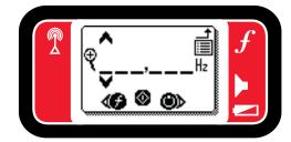
Move all the way to the left of the screen to access a drop-down list stored frequencies. Press the Up and Down Arrow keys <sup>△</sup>♥ to move through the list. When highlighted, press the Select key <sup>◎</sup> to input the frequency.
