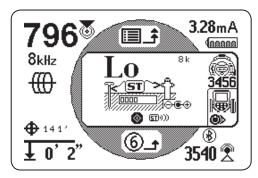
If more than one Bluetooth enabled SeekTech transmitter is present, press the Left Arrow key **1** to cycle through available transmitters. Press the serial number listed below the transmitter icon to identify the specific transmitter you want to control.
