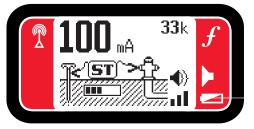
If the display screen shows "Lo," the circuit is open or the unit is unable to draw adequate current for locating. Check your connections and improve the circuit to accurately locate.
