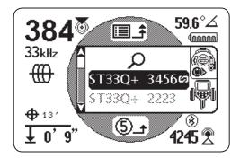
Once a connection is made, the transmitter automatically powers on. When connected, the Bluetooth icon B is visible on both the transmitter's and the receiver's screens. On the transmitter, a chain link image confirms that the two units are connected.
