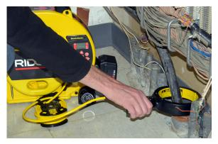
Press the Power key . The ST-33Q+ automatically switches to Inductive Clamp Mode, disables the cable leads, and displays the word "Clamp" on the screen.
