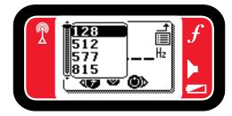
4. Press the Left and Right Arrow keys to move between each digit placeholder and the Up and Down Arrow keys △♥ to increase and decrease the values. The ST-33Q+ adjusts the output frequency as each digit is entered. This auto-adjustment allows the tuning of the target frequency for maximum signal at the receiver. Press the Select key I to save and activate the frequency.
