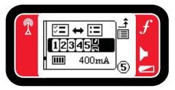
When selected, the Odometer option shows the number of hours each frequency has been used or the number of times each frequency has been selected for actual use. The Odometer option also displays the total time spent in each mode, minimum and maximum voltages encountered, and the amount of time spent at various power levels.
