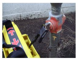
Good contact between the cable lead and the target conductor lowers the resistance of the circuit and produces a stronger tracing signal.
