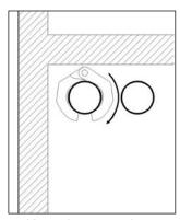
3. Keep the press ring closed and rotate about the fitting until the opening is toward the front.
