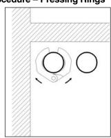
2. ...until the press ring is resting in the groove of the fitting.
