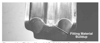
Figure 16 – Fitting Material Build-Up In Press Profile
