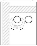
1. Place the press ring around the fitting from the front...
