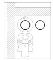
4. Insert the press ring actuator and start the press cycle.
