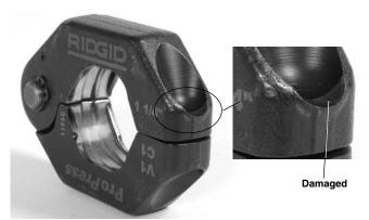
Figure 13 - Damaged Ring Pocket
