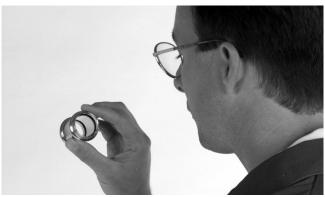
Figure 6A – Inspection of the ProPress Fitting per the Manufacturer's Instructions
