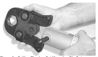
Figure 5 - Pulling The Jaw Set Mounting Pin Out
