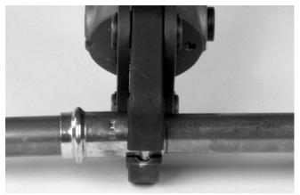
Figure 11 - Jaw Set Square To Fitting and Tubing
