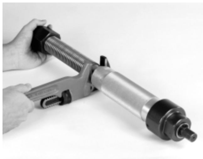
Figure 1 – Assembling Valve Adapter Onto Feed Screw
