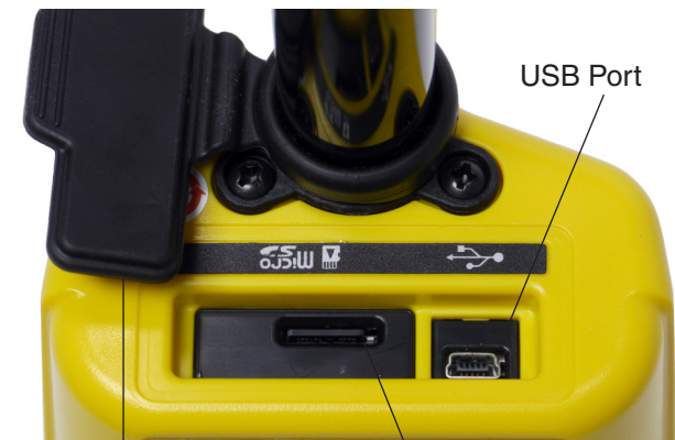
USB Port Cover USB Port Micro SD Card Slot
