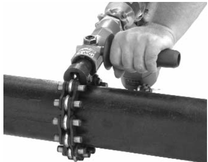
Figure 5 – Operating the Powered Soil Pipe Cutter – Using Impact Tool
