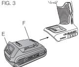
To remove the battery pack from the tool, press the release button (E)
