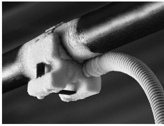
Figure 9 – Freeze Head Frozen to Pipe
