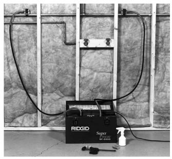
Figure 6 – Two Freeze Plug Application
