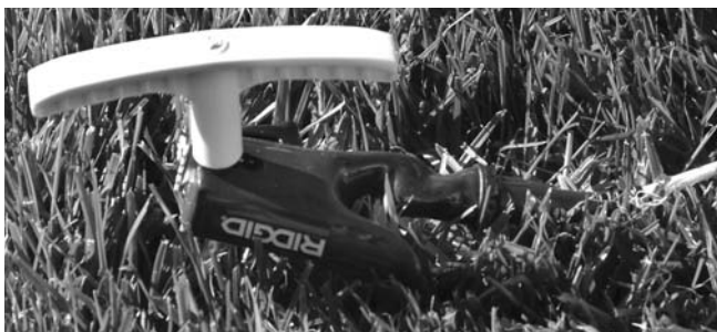
Figure 7 – Attaching Lead To Ground Stake
