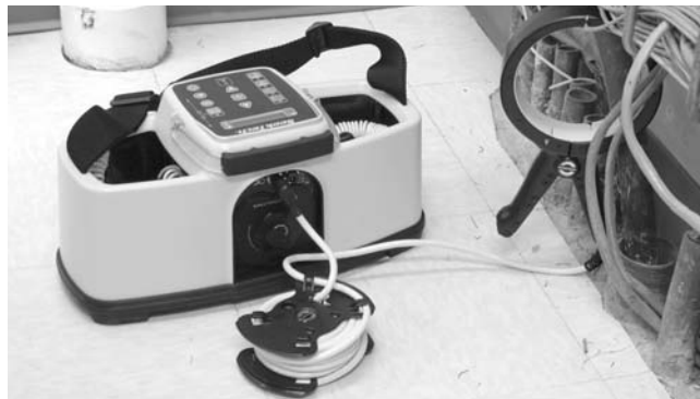
Figure 12 – Inductive Clamp Attached to a Conductor
