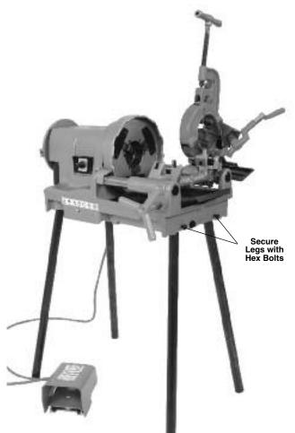
Figure 4 – Threading Machine Mounted On Pipe Legs
