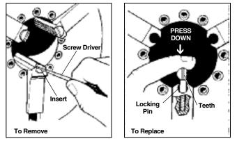
Figure 31 – Replacing Jaw Inserts
