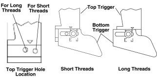
Figure 18 – Adjusting Thread Length
