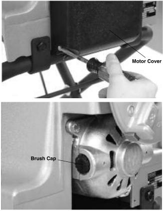
Figure 32 – Removing Motor Cover/Changing Brushes
