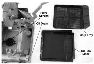
Figure 30 – Filter Screen Assembly
