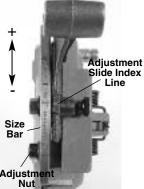
of fitting engagement) as Figure 17 – Adjusting shown on the size bar.
