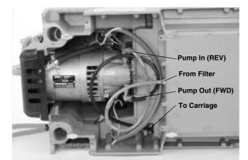
Figure 25A – Oil Pump Connections for Left Hand Threading (Switch in REV)
