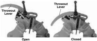
Figure 11 – Open/Closed Position
