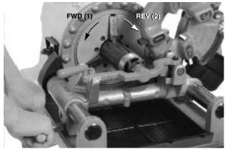
Figure 23 – Reaming Pipe with Reamer, Machine Rotation
