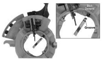
Figure 16 – Inserting Dies
