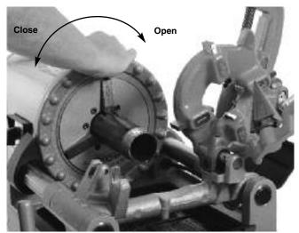
Figure 20 – Chucking Pipe
