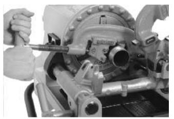
Figure 22 – Cutting Pipe with Cutter
