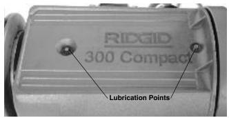
Figure 29 – Lubrication Points
