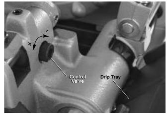
Figure 5 – Adjusting Oil Flow
