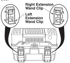
Hook the tab on the bottom of the extension wand clip into the depression in the bottom of the drum. Rotate the clip upwards until the extension wand clip snaps into the slots in the drum, as shown.
