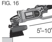
5. Continuously move the tool in a forward and back motion to avoid creating gouges in the work surface. Allowing the tool to rest on the work surface without moving, or moving the tool in a circular motion causes burning and swirling marks on the work surface.
