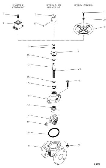
Construction shown is typical of the 2-inch size with flanged end connections and is illustrative only. Construction of other sizes and end connection types vary slightly. See elsewhere on this submittal for specific details.
