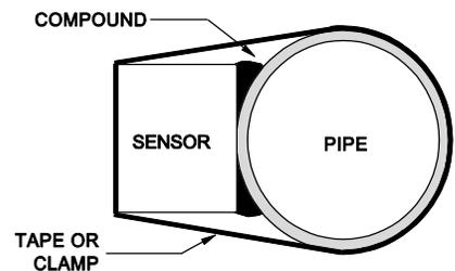
Over time temporary coupling compounds (e.g. Petroleum Gel) may gradually sag away from the sensor resulting in reduced signal strength and finally complete loss of signal. Warm temperatures, moisture and vibration will accelerate this process. Super Lube ® as supplied with the DFM 6.1 (and available from Greyline Instruments or home improvement stores) is recommended for semi-permanent installations.
