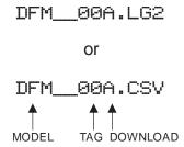
Tag is set according to the Log Site ID entered in the instrument Data Logging menu.
