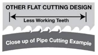
Slower Cutting & More Heat Build-up for Decreased Blade Life  Unique tooth configuration for smoother cuts with less vibration
