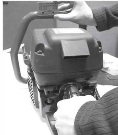
Do not hold the power cutter at maximum RPM for more than 5 seconds.
