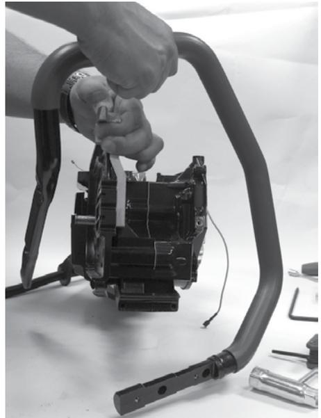
**18. This section covers the removal, inspection and installation of the rear handle.**
