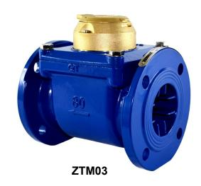
**CONSTRUCTION:** ZENNER Cast Iron Turbine Meters consist of four basic components: The main housing, cover plate, measuring element, and sealed register. The main housing and cover plate are made of epoxy coated ductile cast iron with round flanges, except for the 2" ZTML02 meter which has oval flanges. The measuring element assembly includes the rotor assembly, vertical shaft and a calibration vane which eliminates the need for calibration change gears.
