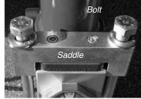
Slowly adjust the pump valve to the neutral position until all hydraulic pressure is on the saddle bolts. Pressure gauge should read zero.
