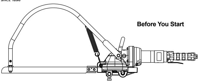
Saw It® pneumatic saws sold prior to the March 2011 introduction of the saw blade guide do not have means to mount the bow spring to the saw. Replacement of the front guide shaft is required. (See Figure 1.) Units sold after March 2011 are prepped. Refer to Saw Guide Installation.
