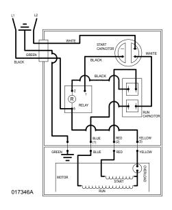
WIRING DIAGRAM FOR MODELS "N202-C" 4/10 thru Current
