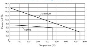
The pressure/temperature chart shown indicates the service limits for the gaskets considering pressure and temperature simultaneously (Tests were performed with nitrogen on 1.6mm [1/16"] thick sheet). The normal curve represents the common usage area for the gaskets while the maximum curve indicates the maximum limits. For applications near or above the maximum curve, contact FNW.
