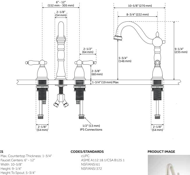
Height: 9-1/4" Height To Spout: 5-3/4" Spout Reach: 8-3/4" Base Plate Diameter: 2-1/8" Handle Length: 2-1/2" Height to Bottom of Handle: 2-3/8" IPS: 1/2" Drain Size: 1-1/2" TAT
