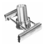
The bucket support and hanger is used for starting a vent at ceiling level. Supports provide proper clearance and automatic positioning. Designed to fit between 16" O.C. joists. Buckets only are available in sizes 9" through 22". Does not act as a firestop. Use firestop (FS). Supports up to 30 feet.
