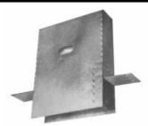
The Type BW attic shield is used on a single-story building or on the top story of a multi-story building for Type BW gas vent. A 26-gauge galvanized sleeve should extend from the top of the ceiling plate into the attic. A Type BW attic shield is required by Los Angeles Code and UMC.
