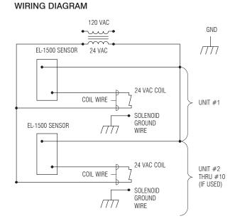
One Transformer serves up to ten (10) OPTIMA Closet/Urinal Flushometers. Specify number of transformers required accordingly.
