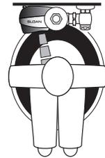
3. When the user steps away, the unit initiates a flush cycle. The unit then automatically resets and is ready for the next user.
