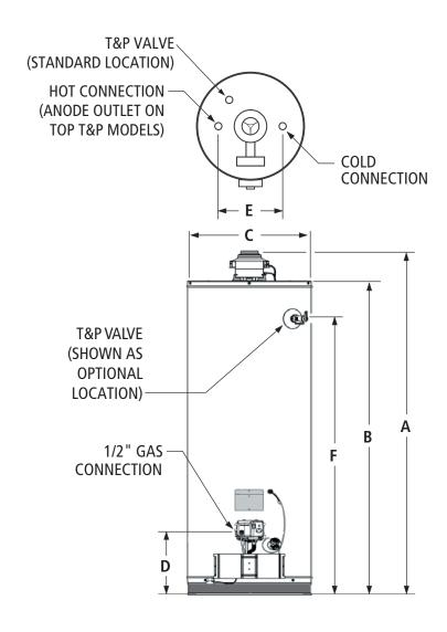
Maximum Hydrostatic Working Pressure: 150 PSI.
