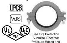
The Figure 772 Rigid Coupling provides a rigid joint by firmly gripping along the circumference of the pipe grooves. Rigid couplings are preferred for dry pipe and freezer applications. Figure 772 Rigid Couplings are a proven dependable method of joining pipe and are an economical alternative to welding, threading or using flanges. It is capable of pressures up to 500 psig (3447 kPa) depending on pipe size and wall thickness when used in fire protection services.
