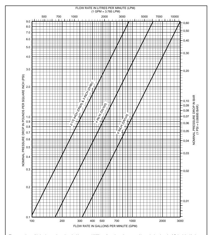
The approximate friction losses, based on the Hazen and Williams formula and expressed in equivalent length of Schedule 40 pipe with C=100 are as follows:
