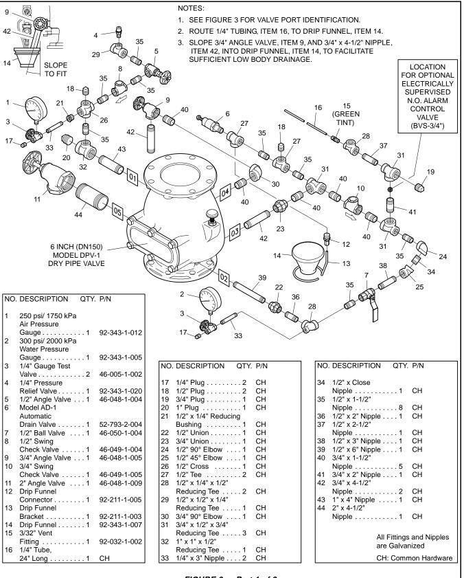
FIGURE 6 — Part 1 of 2 6 INCH (DN150) MODEL DPV-1 DRY PIPE VALVES — EXPLODED VIEW OF VALVE TRIM Page 14 of 20 TFP1020
