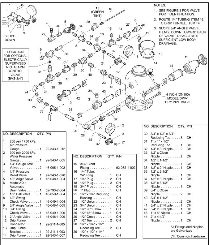
FIGURE 5 — Part 1 of 2 4 INCH (DN100) MODEL DPV-1 DRY PIPE VALVES — EXPLODED VIEW OF VALVE TRIM — Page 12 of 20 TFP1020
