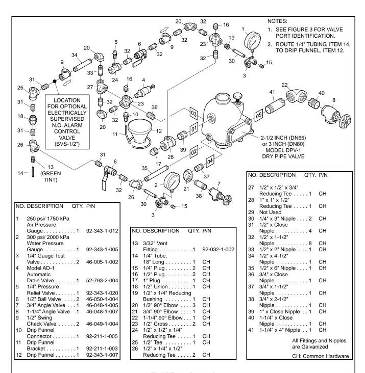
FIGURE 4 — Part 1 of 2 2-1/2 and 3 INCH (DN65 and DN80) MODEL DPV-1 DRY PIPE VALVES — EXPLODED VIEW OF VALVE TRIM — Page 10 of 20 TFP1020
