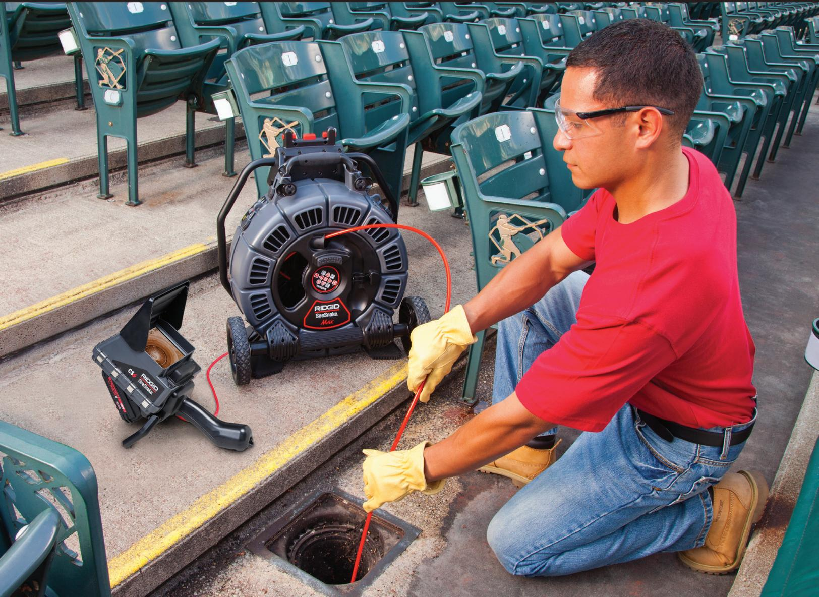
**The rM200 Camera System combines portability with the versatility of the D2 drum series, offering different combinations of push cable stiffness and spring flexibility to tackle any inspection job.**
