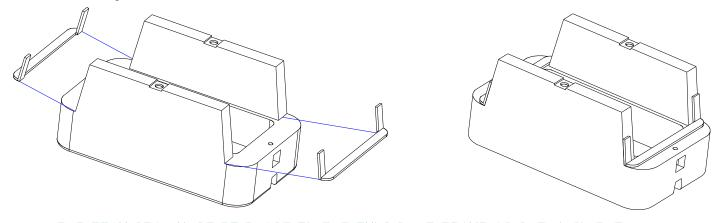
THE FOAM SEAL MUST BE PLACE ON THE OMNI 3 & 5 FRAME AS SHOWN IN THE ABOVE PICTURES BEFORE THE INSTALLATION OF THE COVER AND FRAME. THE FOAM SEAL IS TO PREVENT COLD AIR FROM LEAKING INTO THE VALVE CHAMBER AND CAUSING THE VALVE TO FREEZE.
