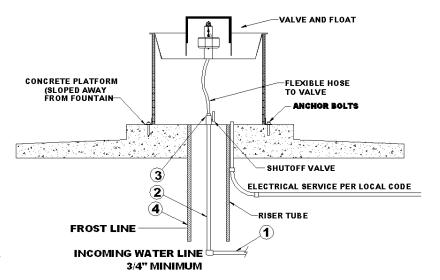
for easier servicing. For optimum serviceability, a stop and waste valve can be installed below frost level to drain water when unit is not in use. Vertical supply line must be centered in riser tube to provide an air space between the line and frozen ground outside of tube. Flush water supply line thoroughly before connection to fountain. Water supplies with foreign material such as sand, rust, etc. may require a filter to keep fountain valve working properly.
