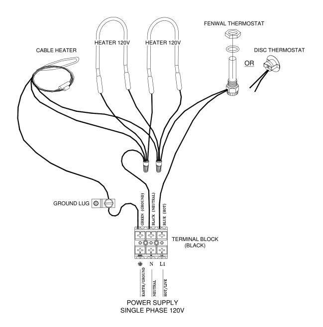
**NOTE:** National/Local electrical codes may require livestock waterers installed in feedlots in open feeding area to be grounded by a separate stranded copper grounding conductor or at least no.6 AWG terminating at a point where the branch circuit receives its supply. Check with local authorities.
