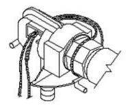
**I. Electrical Connection** - The electrical installation should be made and maintained by a qualified electrician conforming to national and local codes. The 3-wire power to the fountain must be protected by a suitable fuse or circuit breaker with properly sized wire. For wiring connections, see wiring diagram. Wire nuts may be used for the 120-volt and neutral splices.
