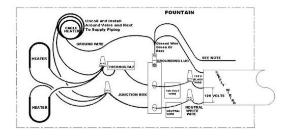
**NOTE:** National/Local electrical codes may require livestock waterers installed in feedlots in open feeding area to be grounded by a separate stranded copper grounding conductor or at least no.6 AWG terminating at a point where the branch circuit receives its supply. Check with local inspection authorities.
