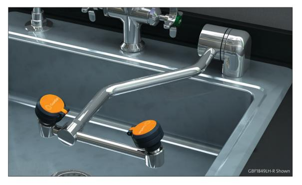
**Application:** Barrier-Free, AutoFlow™ eyewash for mounting on counter. Eyewash outlet assembly is lowered and extended to permit access by wheelchair user. ADA compliance is dependent on 27" knee clearance under counter and 34" maximum counter height. Spray heads swing down from storage to operational position, activating water flow. Available in a variety of spray head configurations to minimize obstructions at a sink.
