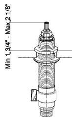
4. The head valves height on the sink should be between min. 1 3/4" and max. 2 1/8" (recommended height 1 7/8").
