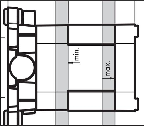
To insure correct fit of the showerhead, the outside surface of the finished wall must fall between the "min" and "max" markings on the plaster shield.
