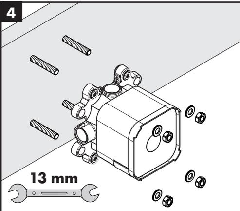
Install the rough with the washers and nuts.
