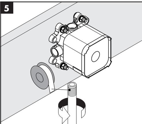
Wrap the threads on the pipe using plumbers' tape.
