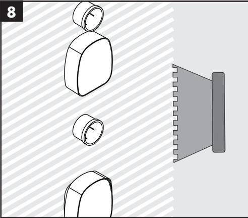
Spread adhesive on the wall around the rough(s).
