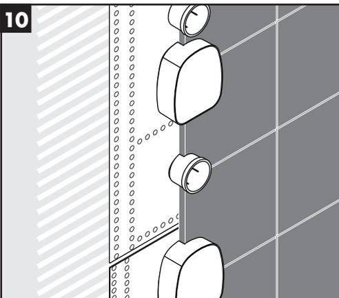
Install the tile or other finished wall surface over the gasket and against the rough installation box.
