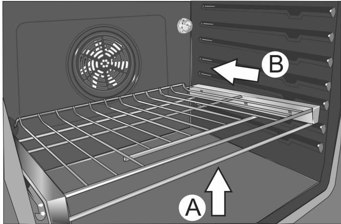
3. The back of the telescopic rack drops into place.
