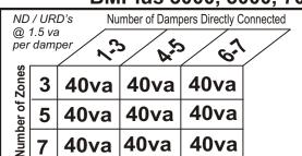
Use Class 2 UL Listed 1585 Inherently current limiting transformers only!
